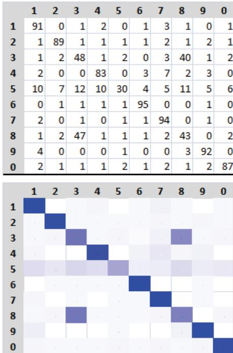
**Figure 2. Representations of confusion matrix for a handwritten digit classification task. (top) standard confusion matrix; (bottom) heat-map confusion matrix. It is much easier to identify underlying patterns in the visual representation; 3 and 8 are often misclassified as each other and 5 is misclassified as many different numbers.**
