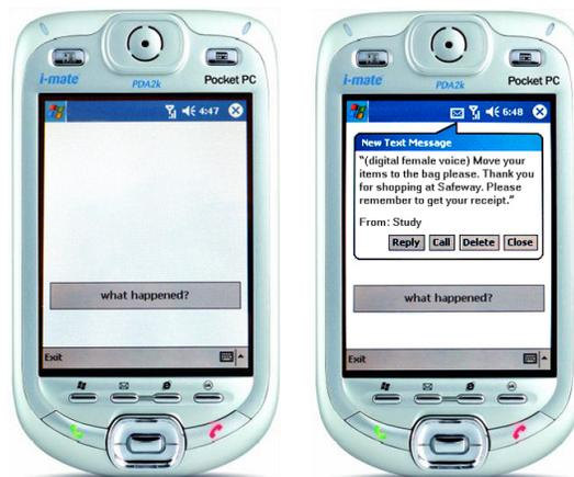
**Figure 3:** The Scribe4Me system caches 30 seconds of audio and sends it to an experimenter for transcription when the user presses the "what happened?" button (left). When the experimenter completes the transcription, it is displayed (right) [24].
