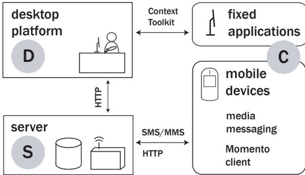
**Figure 2:** System architecture. The desktop platform (D) and server (S) communicate with clients (C) via SMS/MMS, HTTP, or the Context Toolkit. Study data is stored for later analysis or retrieval via the web.
