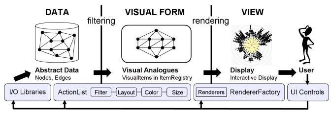
**Figure 2.** The prefuse visualization framework. Lists of composable actions filter abstract data into visualizable content and assign visual properties (position, color, size, font, *etc*). Renderer modules, provided on a per-item basis by a RendererFactory, draw the VisualItems to construct interactive Displays. User interaction can then trigger changes at any point in the framework.
